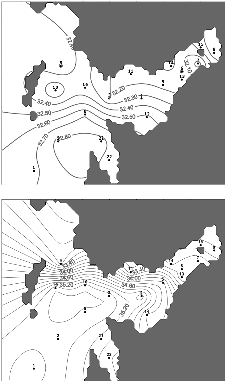
Figure 4.29: Measured surface and bottom fields of salinity in the ria on cruise 4po11.
