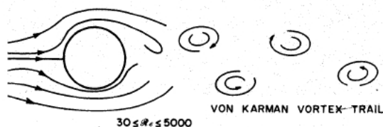
Figure 1.2: Flow past a cylinder for 30 < \text{Re} < 5000 [2]
