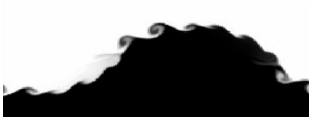
Figure 3: Cross-stream convective rolls along interfacial wave [1]
