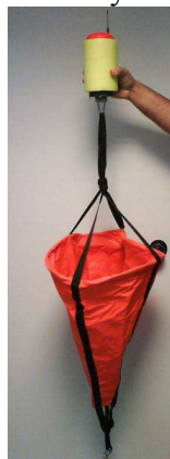
Figure 3 – drifting buoy with underwater drogue
