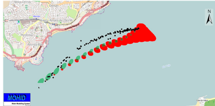
Figure 5 - Buoys survey, on 4th August 2010: black dots - measured buoys position along time; red polygons – particles from backward model run; green semi-transparent polygons – particles from forward model run
