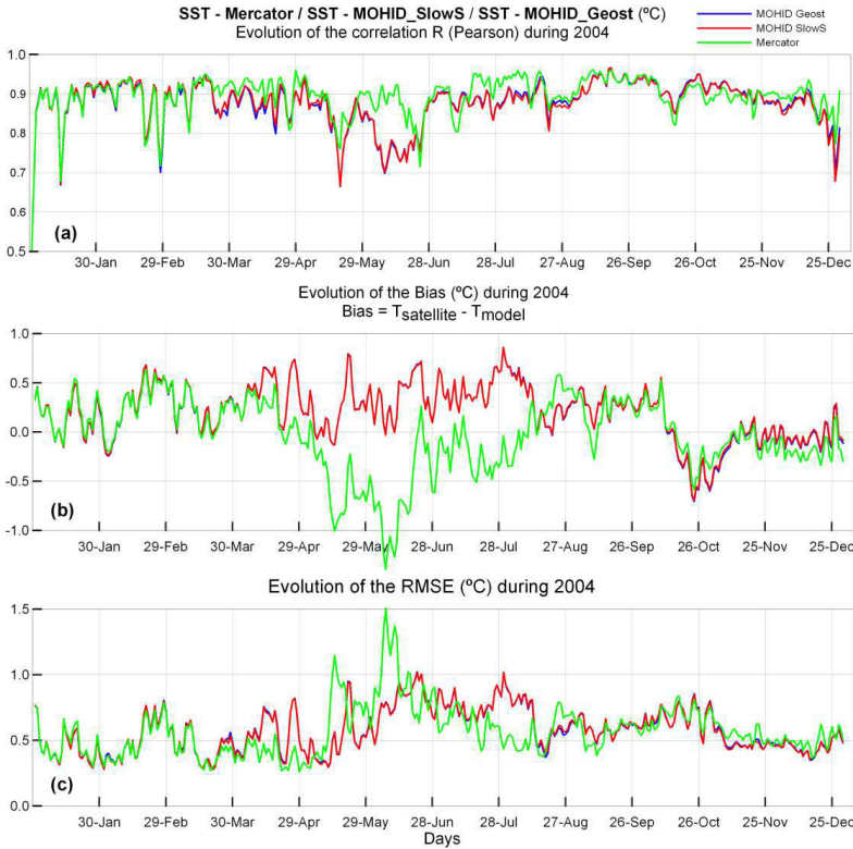
Figure 5. One year comparison between Microwave SST and the results of the two simulations (also for Mercator solution): (a) Pearson correlation coefficient; (b) Bias; (c) Root mean square error.
